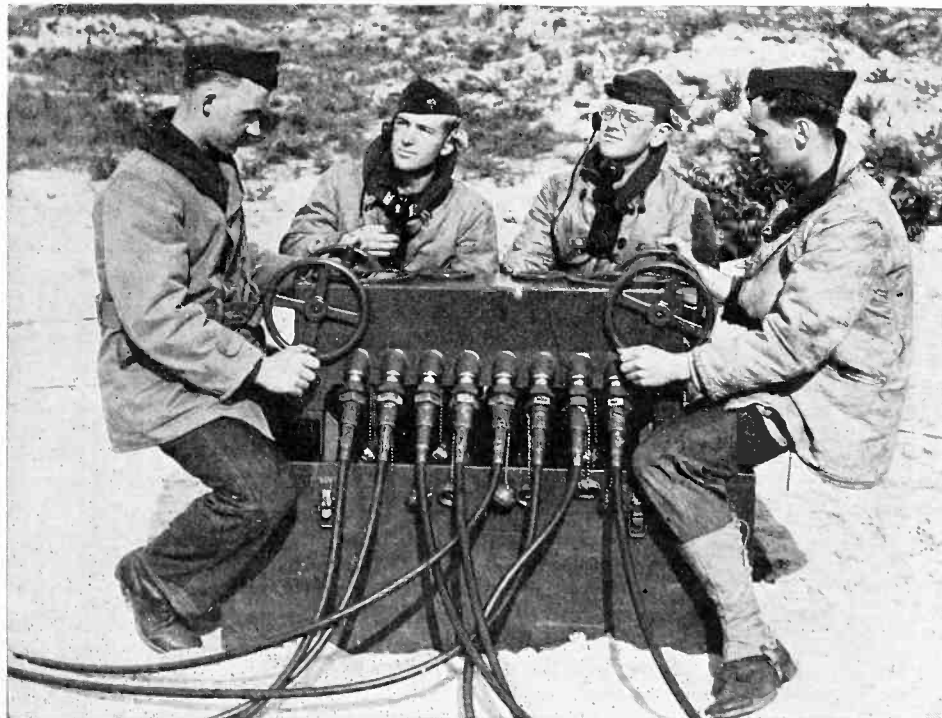
This synchronizer is used during firing practice of 50-calibre heavy machine guns by the 62nd Coast Artillery at Fort Totten, N. Y. The two men with the headsets receive information from the battery commander stationed some distance away, on matters of wind velocity and leads. This information is mechanically transmitted through adjustments on the panel and impulses are sent through the appropriate cables in the foreground which automatically adjust the sights of the gun
