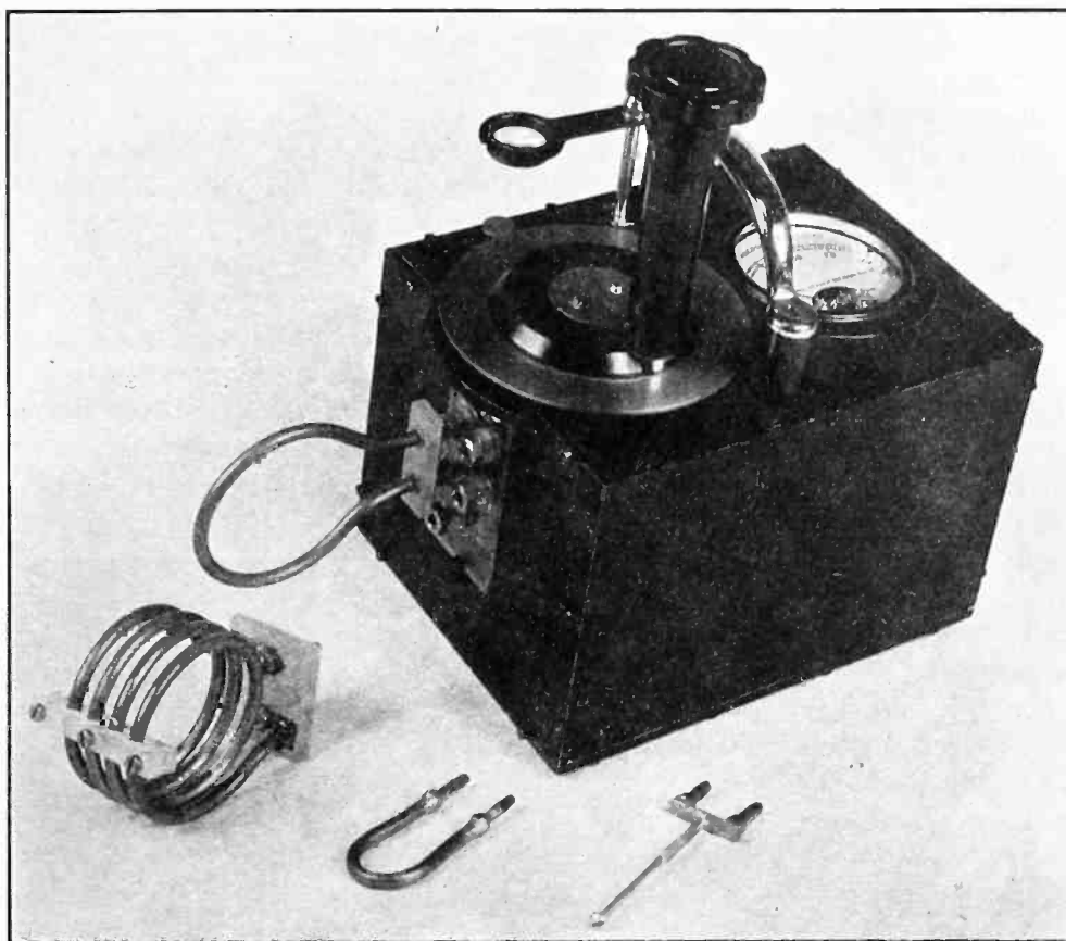
Fig. 1—External appearance of the meter. A rugged two-section capacitor is used with the coils shown to cover the 30 to 340 megacycle range
