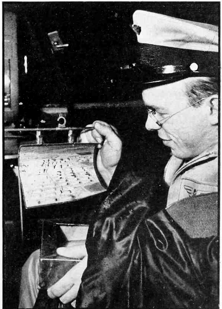
Fig. 4—Above, the picture is transmitted at the rate of 8 square inches per minute or about 8 minutes for a picture of standard telegram size, 8 3/4 by 7 inches. The signal is applied to the f-m transmitter at the microphone input terminals
